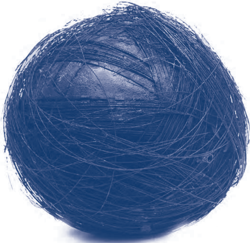
Fi 103 compressed air container with surrounding wire coil
