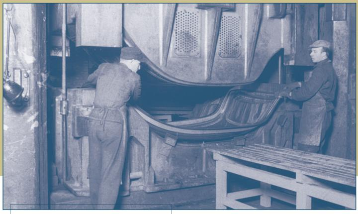
Workers remove the roof of a saloon car from the press.
