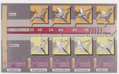
How the dual-airbag system operates
