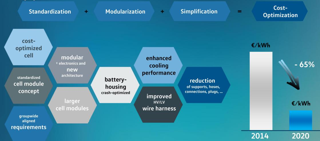
MEB battery: Development focus on cost reduction, flexibility and robustness
