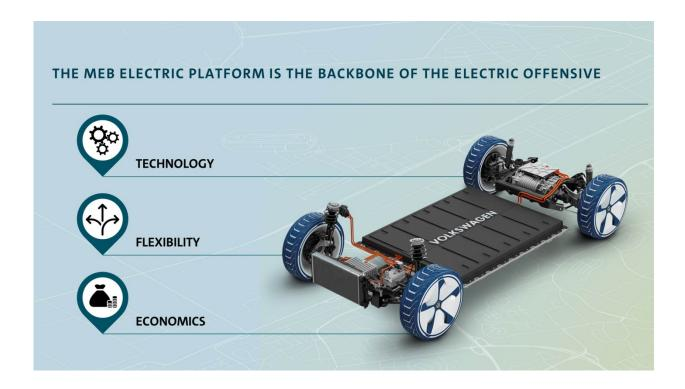
The ID.3 is the first vehicle based on the Modular Electric Drive Toolkit I mentioned previously. The MEB has been developed as an all-electric platform. It makes optimum use of the latest technologies – in terms of performance, space and digital offerings. The MEB means we can achieve ranges in excess of 550 kilometers (in accordance with WLTP).
