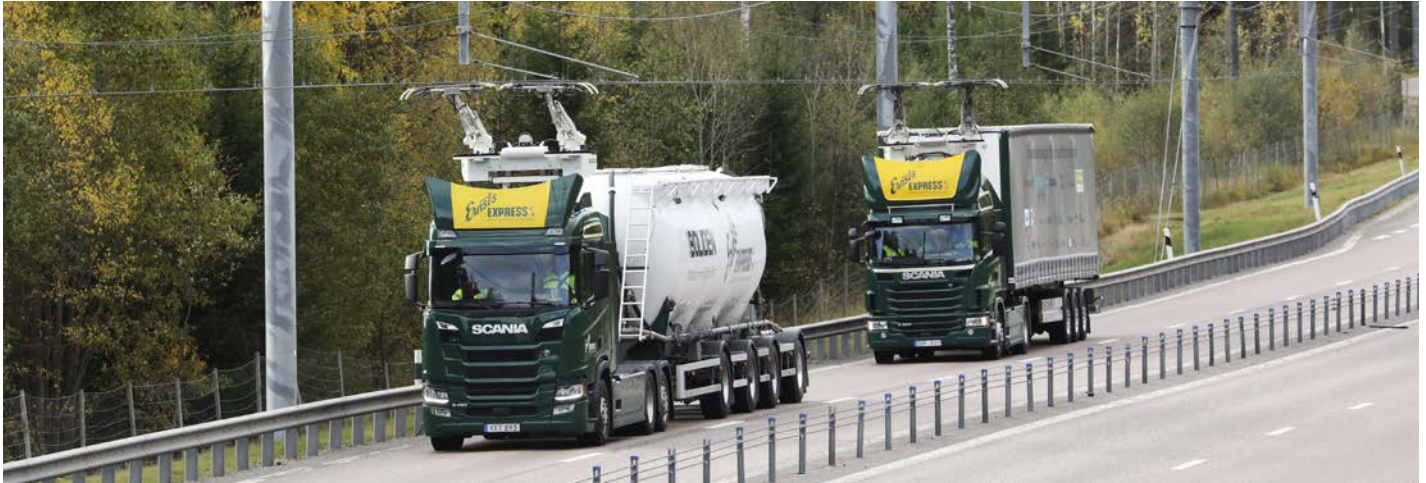
In the world's first electric road project, two electrically-powered Scania trucks drive a route in open highway traffic, using conductive technology developed by Siemens.
