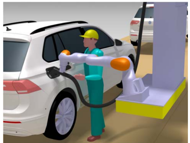
Adaptation of the AdBlue filling adapter for use with a lightweight robot
